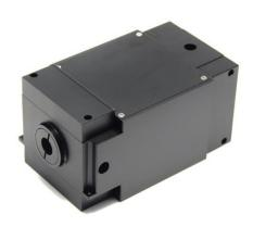
The IHPF series high-power free-space optical isolators are engineered for 100-W-class, single-polarization laser systems and use Agiltron's proprietary configuration with advanced thermal-management technologies to achieve efficient heat removal under high optical radiation. These dual-stage isolators provide >45 dB isolation, with power-handling capability determined by aperture size; beam expansion and collimation are required to match the beam to the aperture and reduce power density.
